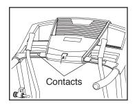
To measure your heart rate, stand on the foot rails and hold the metal contacts on the handrail. Avoid moving your hands. When your pulse is detected, a heart symbol in the lower right display will flash each time your heart beats, one or two dashes will appear, and then your heart rate will be shown. For the most accurate heart rate reading, continue to hold the contacts for about 15 seconds.
